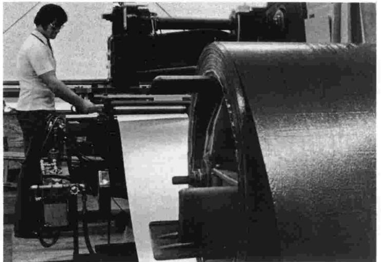
Copper for the Zappone copper shingles arrives at the Spokane factory 26,000 pounds at a time in 16-inch wide, 2,000-pound coils of strip, as seen here.
